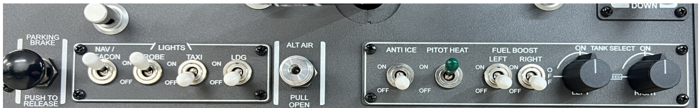
Parking Brake Lights, Alt Air, Anti-Ice, Pitot Heat, Fuel Boost Pumps and Fuel Tank Selectors
