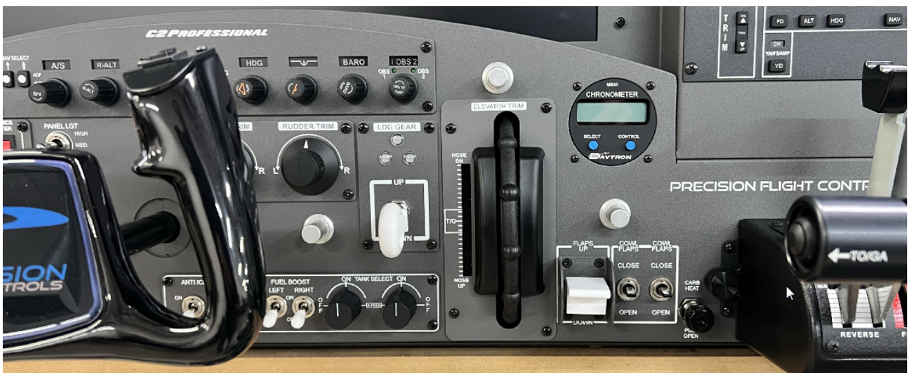
Elevator Trim Wheel, Flaps Switch, Cowl Flaps and Digital Clock
