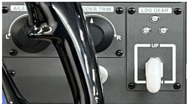
Landing Gear Switch with Gear Position Lights
