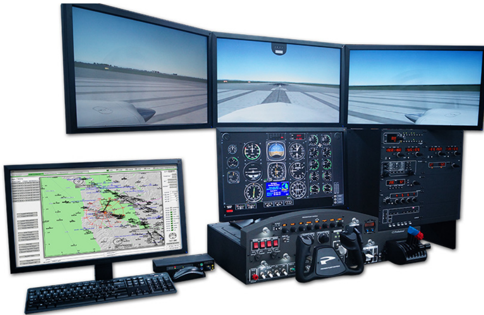
CR12 Shown with 3 LCD Monitors, Instrument Screen, Avionics, IOS Monitor, KVM, Keyboard and Mouse
