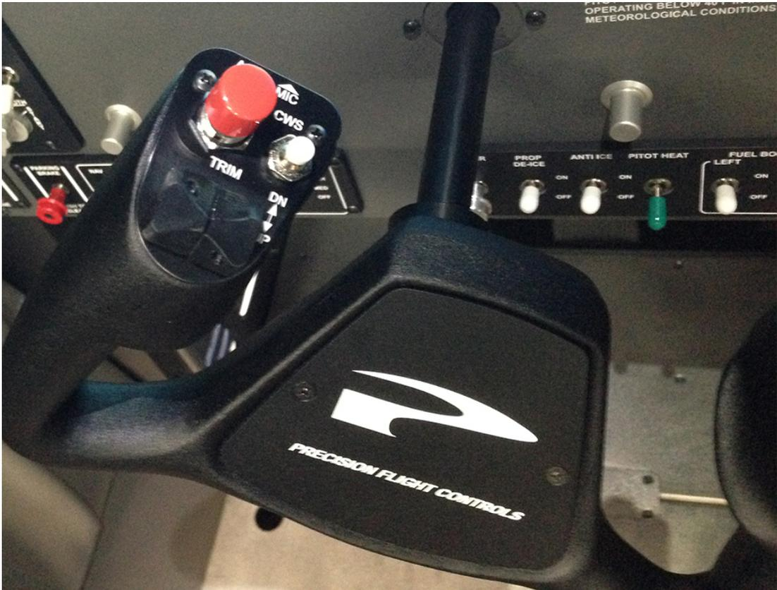
Enhanced Yoke Controls with Elevator Trim, CWS, A/P Disconnect Switches
