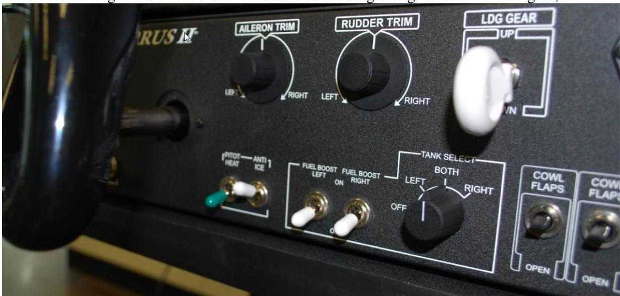
Close up of (partial) Switches, Trim Rudder and Aileron Trim Controls, Fuel Selector, Fuel Boost Pumps Cowl Flaps and Landing Gear
