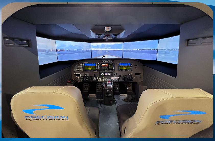
Five 40" 4k monitors are integrated into the flight deck. Both the left and right monitors are tucked back into the visual enclosure providing a "look "over your shoulder view" for pattern work while keeping the runway in site. Because of the wide viewing capability you can practice demanding procedures in all types of weather conditions including: ILS, RNAV, NDB, Circle to Land, LOC and more.
