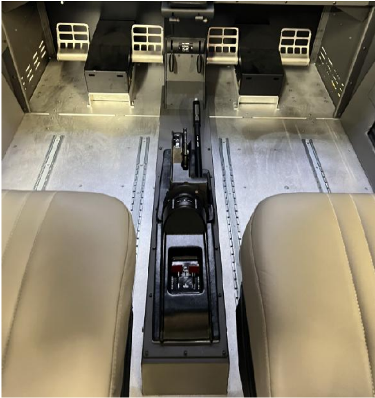
Piper Seminole Center Console Elevator Trim Rudder Trim Aileron Trim Fuel Selectors Flaps Lever
