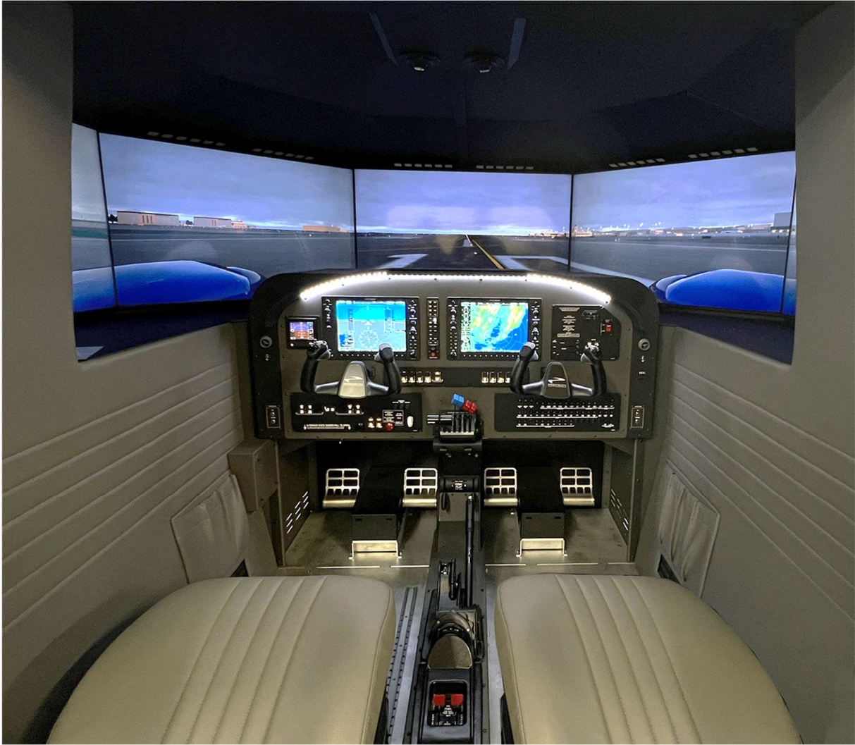
GTX MAX, GTX MAX PROMOTION Flight Deck (Shown in Piper Seminole Configuration) Note: All Panels are interchangeable with the Archer Panels
