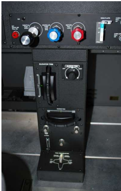
GTX MAX / GTX MAX Promotion Center Flight Console Elevator Trim, Rudder Trim, Aileron Trim, Cowl Flaps and Fuel Tank Selector
