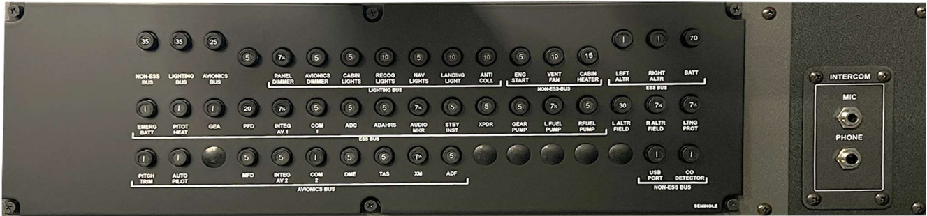
Circuit Breaker and Intercom (Piper Seminole)
