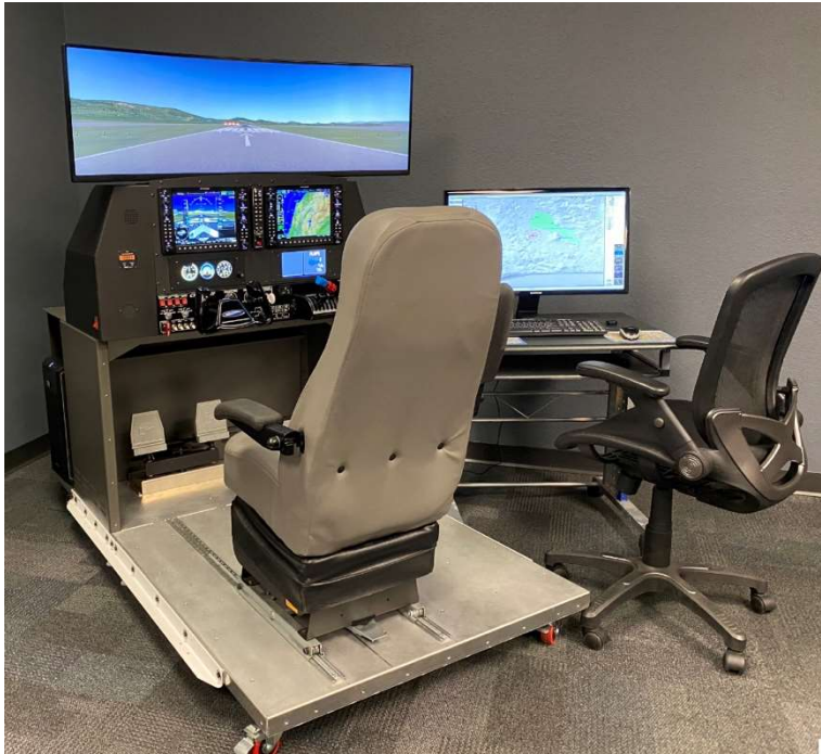
GTX shown with Single Screen Visual Display and Instructor's Station With Yoke
