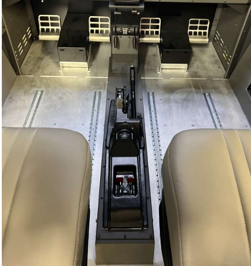
Piper Seminole Center Console including Elevator Trim, Rudder Trim and Fuel Selectors
