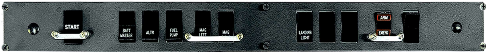
Piper Archer Overhead Panel
