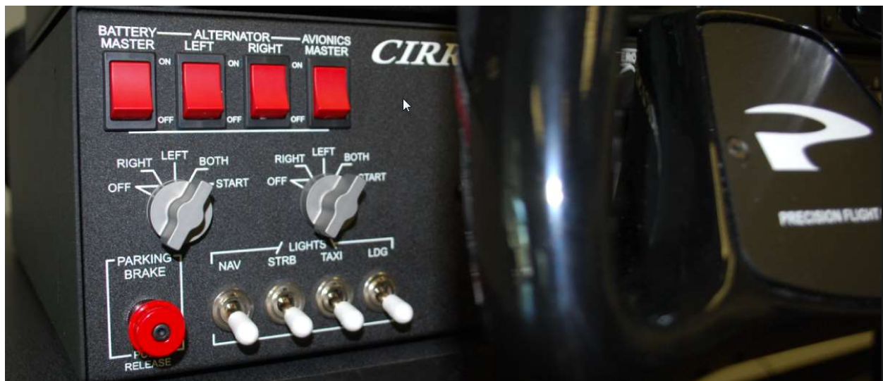
Close up of Magneto Switches, Battery, Avionics and Alternator Switches and Light Switches The Master/Magneto Switches Can Be Used to Start Single Engine and Multi-Engine, Aircraft
