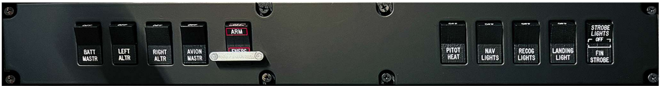
Battery master and Light Panel (Piper Seminole)
