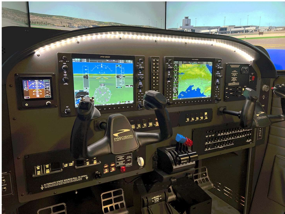
Piper Seminole Instrument Panel including PFD, MFD, Audio Panel and Standby Instrument
