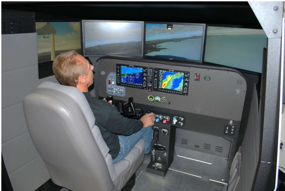
GTX MAX / GTX MAX Promotion Shown with Integrated Five Screen Visual System
