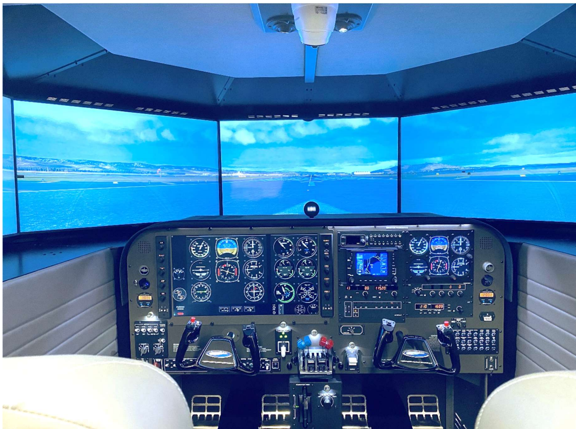
Two hundred Degree High Resolution Visual System With Detailed Scenery
