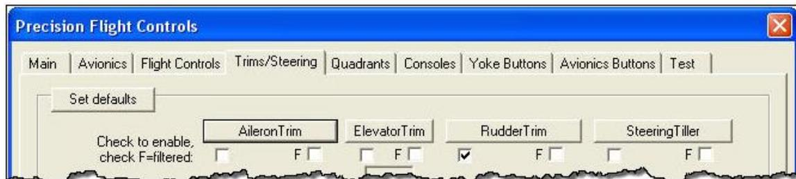
6. Enable the **Rudder Trim** and turn it left to right and see if the indicator is responding.
